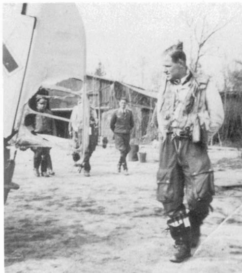
Hptm. Müncheberg looks over Oblt. Wutz Galland's Focke-Wulf after combat on the afternoon of 25 April. This level of damage would not have been reported to Berlin; a rudder could be changed easily out on the Gruppe flight line. ( Van Boxem via Vanoverbeke )
