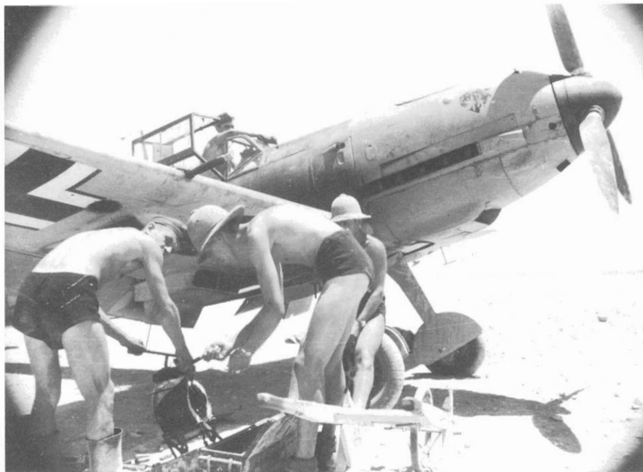
Armorers are apparently working with a magazine for a MG FF wing cannon. The desert sand is rapidly eroding the airplane's "Red Heart" Staffel emblem – Libya, mid-1941. ( Bundesarchiv-Bildarchiv )
