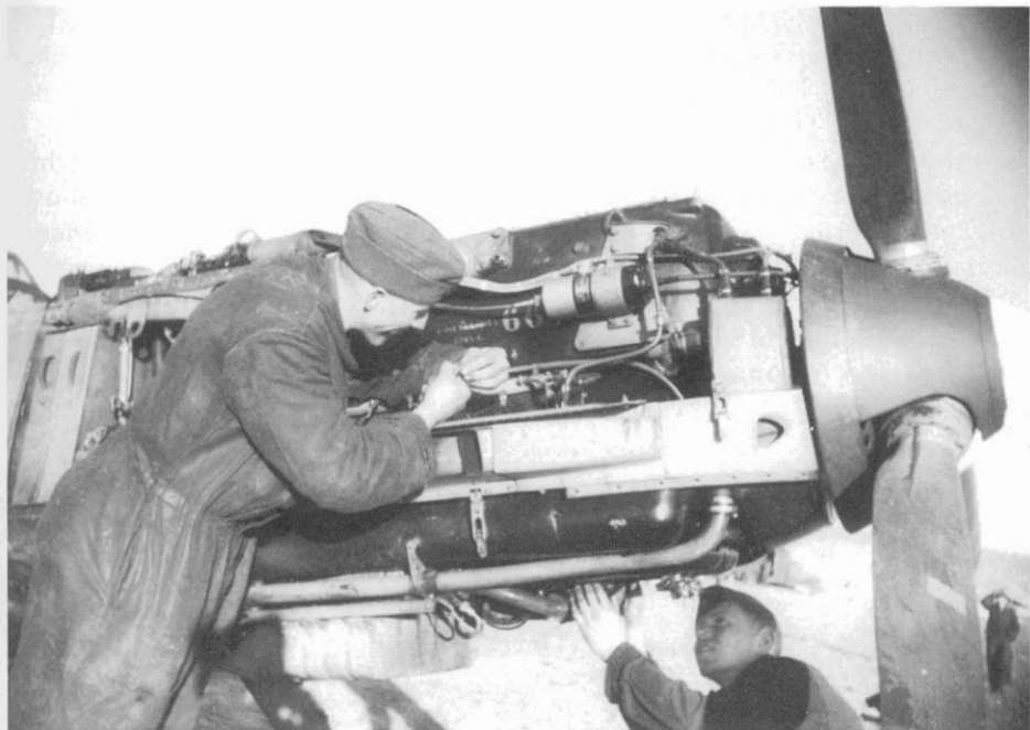
A DB 601N engine is worked on soon after the unit's arrival in Sicily in February. ( Bundesarchiv-Bildarchiv )
