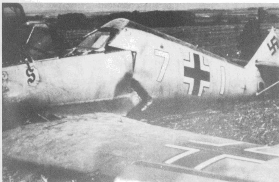
Lt. Bürschgens bent his Bf 109E-1 "white 7" (W.Nr. 4495) while force-landing on Caffiers after combat over England on 11 August. The weakest point of the Messerschmitt fighter's fuselage was right behind the cockpit. ( Wermann )
